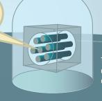
The fourth barrier is enclosed within the airtight reactor building. The building has concrete walls at least four feet thick.
